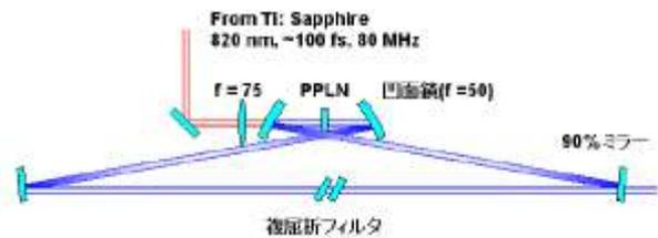
Fig.1: Our concept of a Ti: Sapphire pumped SOPO. We adopted four-element ring cavity and R=90% output coupler.
