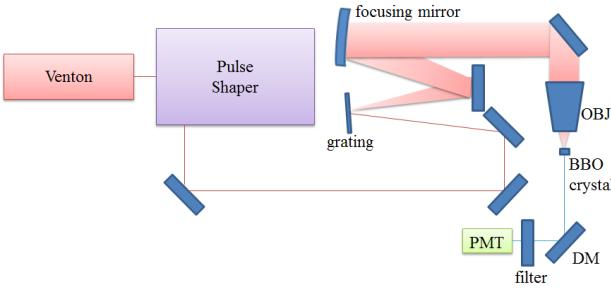
Fig. 1. SSTF experimental setup. Venteon: mode-locked Ti:Sapphire laser. OBJ: objective lens (Olympus UPLSAPO 40X). DM: dichroic mirror. PMT: Photomultiplier tube.
